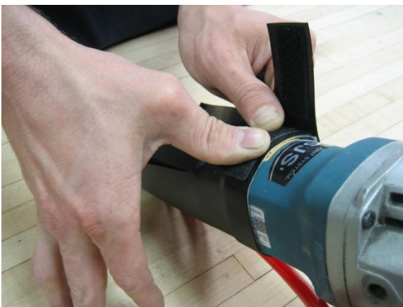
FIGURE 5 – Spray Skirt Installation, #3
