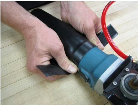
FIGURE 3 – Spray Skirt Installation, #1
