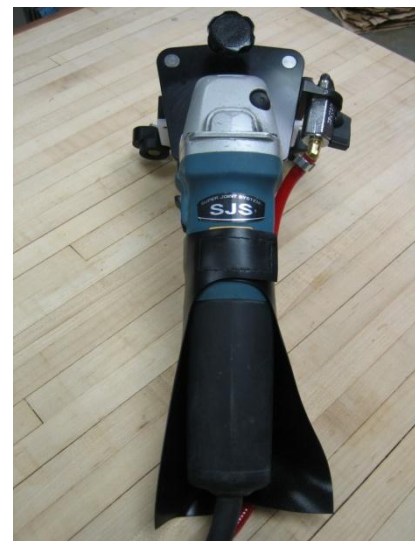
FIGURE 6 – Spray Skirt Installation, #4
