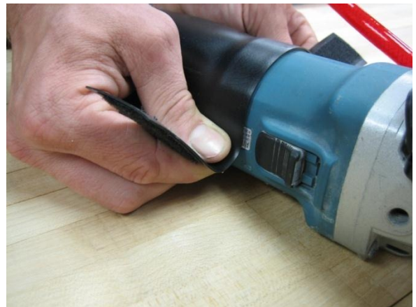
FIGURE 4 – Spray Skirt Installation, #2
